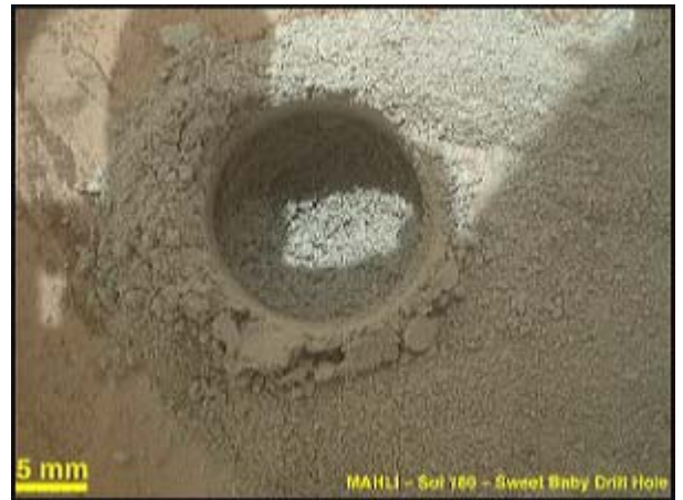
First test drill completed on Feb 6, 2013. Hole is 0.65 inches in diameter. It is interesting to note that the color of the rock powder is grey as opposed to the oxidized red color of the surface rock.
