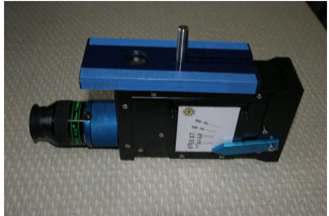
Lhires Lite: Notice gnome on top with the home-made etalon holder (blue taped on sides) attached at the gnome.
