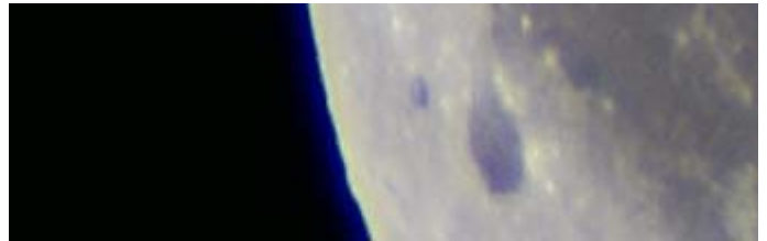
Above: Moon limb with 1987 vintage, 75mm "ED" (taken 6/09). Note the blue fringe. Below: Moon with the AT72mm (6/10). No chromatic aberration. Both images are cropped close-ups to reveal any color.
