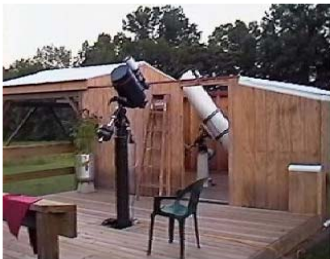
A pier on the deck was for the 10" Meade SCT purchased from the CVAS. It was to be dedicated to astro-imaging.
