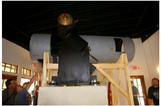
Norm Oberle's 25" Newtonian being refurbished.
